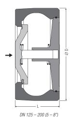
Non-Return Valve for Sandwiching between Flanges PN 6/10/16, ASME Class 125
