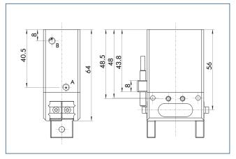
The mechanical gripping force maintenance device ensures that a minimum clamping force will be applied even if there is a drop in pressure. This acts as closing force in the AS / S version, and as opening force in the IS version. Besides this, the gripping force maintenance device can be used to increase the gripping force or for single actuated gripping.
