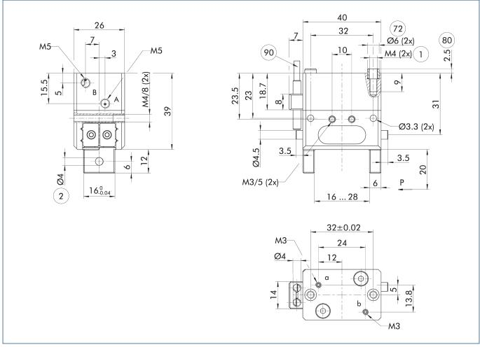
The drawing shows the basic version of the gripper with open jaws, without dimensional consideration of the options described below.
