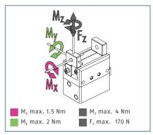
The indicated moments and forces are statical values, apply for each base jaw and should not appear simultaneously. Loads may additionally occur to the moment produced by the gripping force itself.
